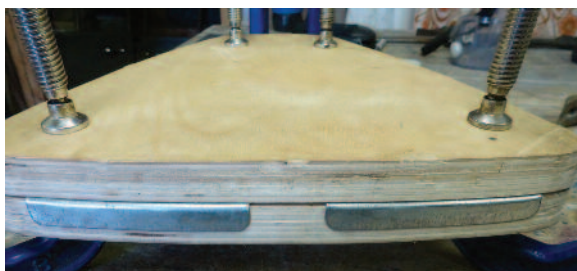
Picture 6. Internal baffle plate edges hammered over.
