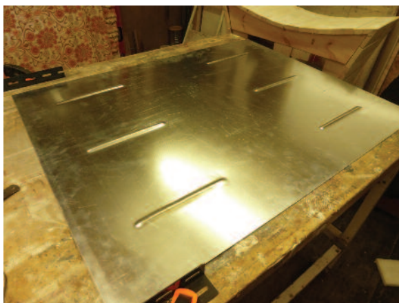
Picture 14. The completed tank side indents
