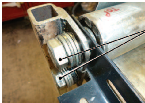
Picture 18 Roller tube pivot bolts close-up
