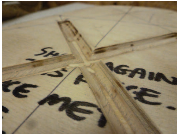
Picture 3. Close up of indents on plywood pattern.
