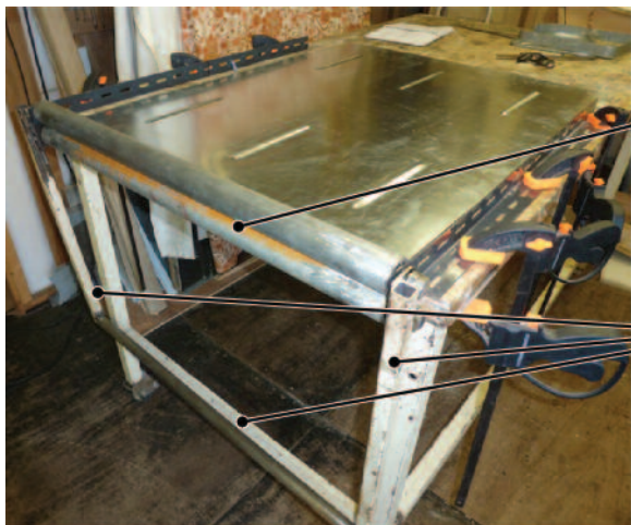
Picture 15. Roller jig clamped to bench.
