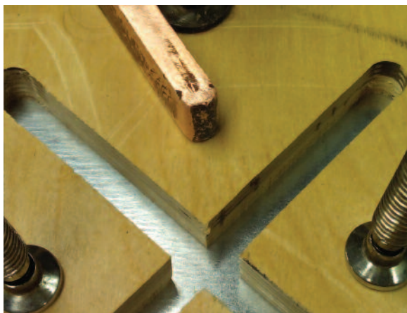
Picture 9. Close up of modified patterns for end plate indent forming.
